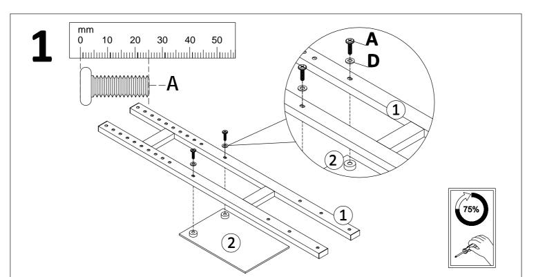
Note: Do not fully tighten until assembly is completed .
