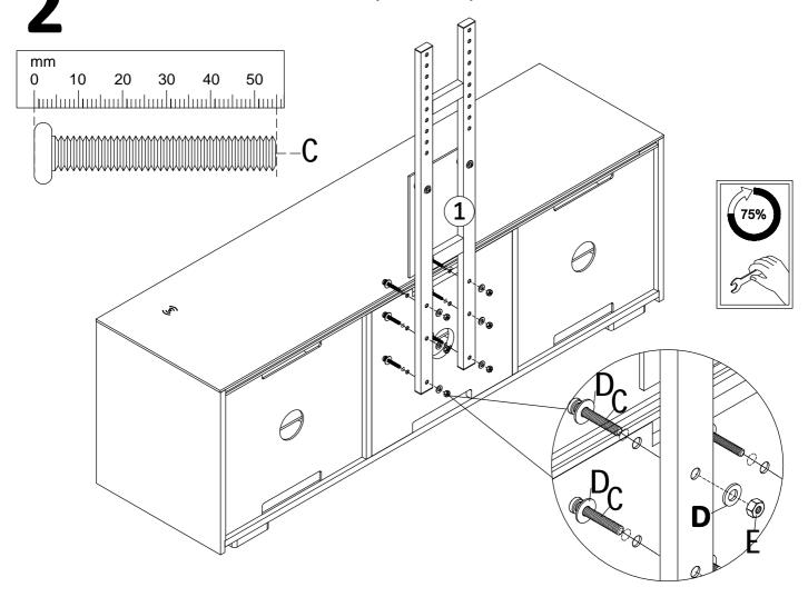
Note: Do not fully tighten until assembly is completed .
