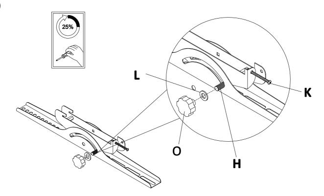
Note: Do not fully tighten until assembly is completed .
