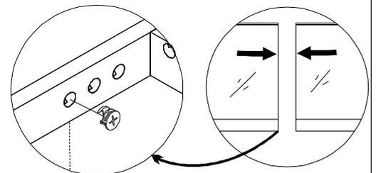
Position base to the left or right when two units are combined to make one large central base
