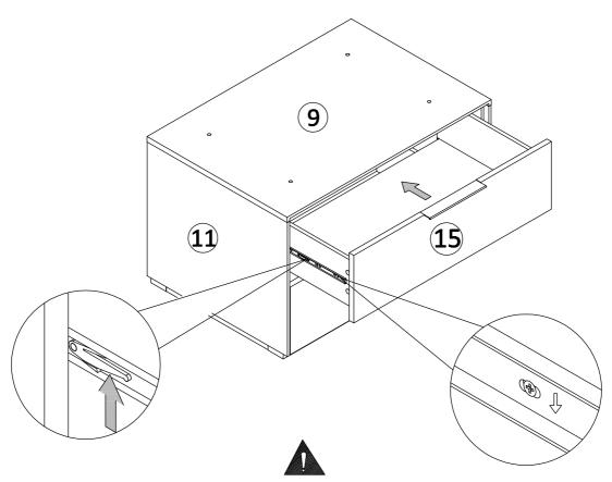
The gap between the drawers can be altered by loosening the screw and moving the runner up or down.
