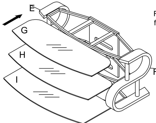
Fully tighten fittings before fitting glass.
