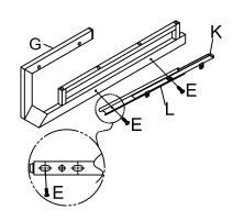
Fit runners to metal brackets using bolt "E",start by sliding the runner until it is fully extended then proceed to secure rear of runner first,making sure you use the hole furthest back,Then close the runner and secure the front using the hole that is now aligned
